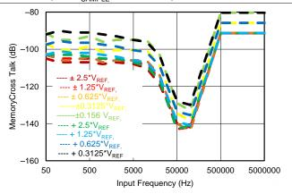
Figure 57. Memory Crosstalk vs Frequency
