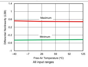
Figure 16. DNL vs Temperature
